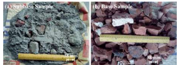
Figure 5 (a) Sub-base and (b) Base samples collected from Kaliganj, Satkhira
